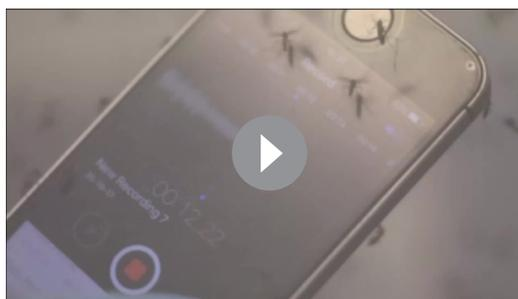
**Video 3.** Demonstration of how to record sound from a mosquito in free flight, at the moment of take-off, using a mobile phone.
