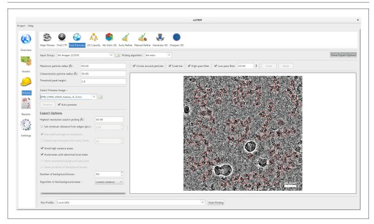
**Figure 3.** Particle picking panel of the *cis*TEM GUI. The panel shows the preview mode, which allows interactive tuning of the picking parameters for optimal picking. The red circles overlaying the image of the sample indicate candidate particles. The picking algorithm avoids areas of high variance, such as the ice contamination visible in the image.
