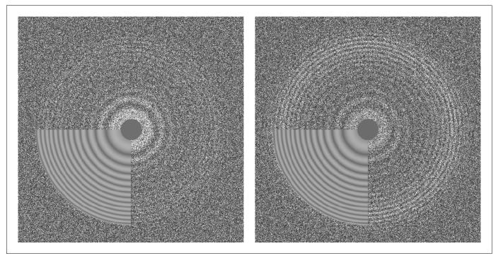
Figure 2. Thon ring pattern calculated for micrograph '0000' of the high-resolution dataset of β-galactosidase (*Bartesaghi et al., 2015*) used to benchmark *cis*TEM. The left pattern was calculated from the average of non-exposure filtered and aligned frames while the right pattern was calculated using the original movie with 3-frame sub-averages. The pattern calculated using the movie shows significantly stronger rings compared to the other pattern.
