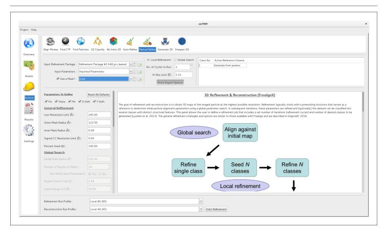
**Figure 4.** Manual refinement panel with Expert Options exposed. Most of the parameters needed to run FrealignX can be accessed on this panel. The panel also allows application of a 3D mask, which can be imported as a Volume Asset. DOI: https://doi.org/10.7554/eLife.35383.005
