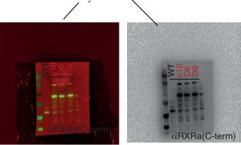
Original uncropped image for anti-RXR $\alpha$  (C-term) blotted signal for RXR $\alpha$  endo clones.
